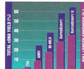
Comparison of Reverse Transcriptases using 1 µg of a 7.5-kb RNA Template.
